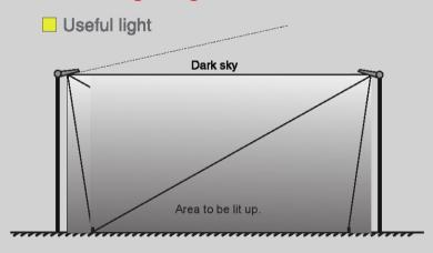
LED Floodlight is specially designed for sports fields, minimizing loss of light and light pollution.
