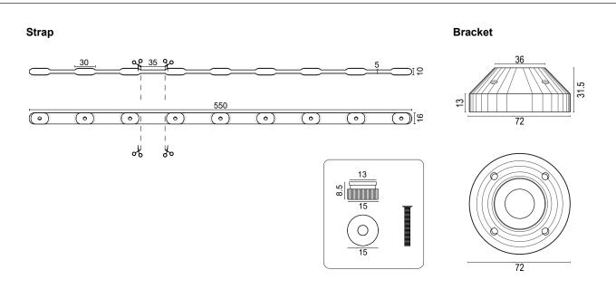
This product can be used for trees with a max Ø200mm trunk. In order to use the strap for smaller size of trees you can cut the rubber belt to match the size of the trunk accordingly.
