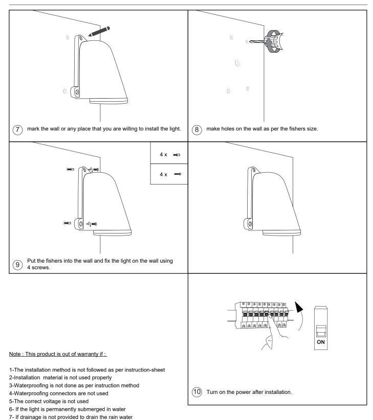
Note : To prevent any risk while doing installation of this product an electrical engineer need to install / supervise installation team.
