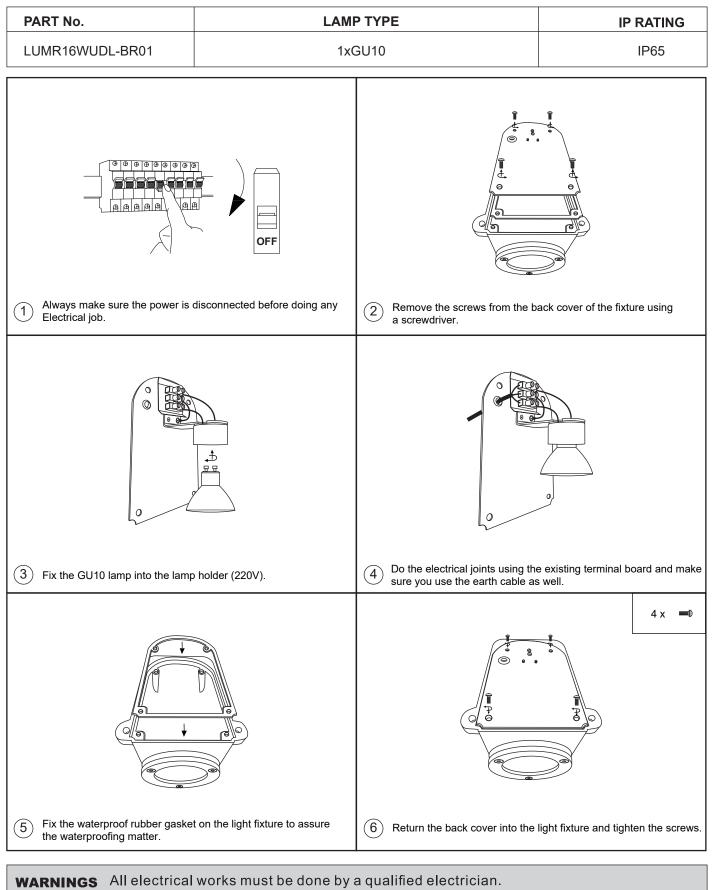
Turn off electrical power to all affected circuits before installation or servicing. For any technical support contact LUMO® experts in info@lumo.ae
