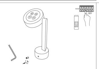
Turn Off the power and remove screws from both side take out the fixing bracket.
