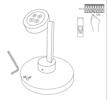
6. Insert light into bracket and tighten the screws from both side with allen key.
