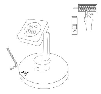
6. Insert light into bracket and tighten the screws from both side with allen key.
