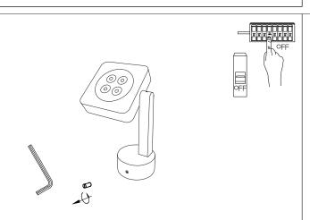
1. Turn Off the power and remove screws from both side take out the fixing bracket.
