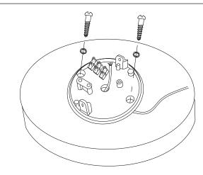
4.Fix the bracket on desired surface using the screws.
