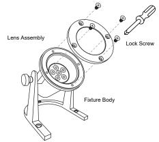
Install Lens Assembly - Place the lens assembly back onto the fixture body and secure with lock screws. Tighten until snug with a screwdriver.
