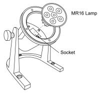
Install Lamp - Insert the lamp with the correct wattage and type as marked on the fixture label.
