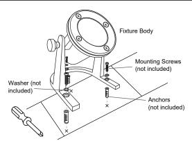
Mount Fixture Body - Postion the fixture body in a desired location. Using the slots on the fixture base, mark the two mounting points. Using the marks, drill holes and insert the anchors. Place the fixture body onto the anchors. Pass the washers over the mounting screws and thread the mounting screws into the anchors to secure the fixture body. Hand tighten until snug with a screwdriver.
