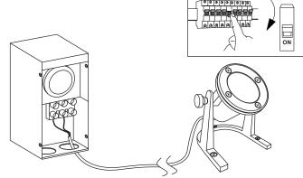
Wire Connection - Lay out the supply cable to the transformer. Strip both of the leads from the luminaire pigtail. Connect the leads from the luminaire supply cable to the transformer (sold separately). Turn on the power after installation.
