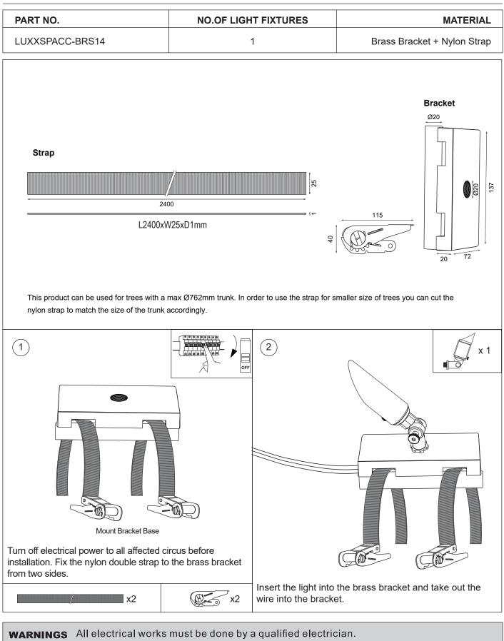
Turn off electrical power to all affected circuits before installation or servicing.
